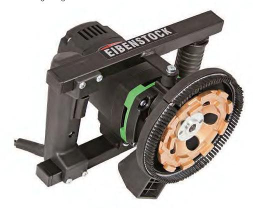
**Type:** EBS125.4 Disc size: 125mm/5" Voltage: 110v **Input: 1500w** Bore: 22mm Spindle Size: M14
